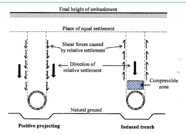
The reduced load on buried utilities using induced trench installation method and EPS geofoam has been demonstrated in research conducted using both laboratory simulations<sup>1</sup> and through ongoing monitoring of utility line installations.
